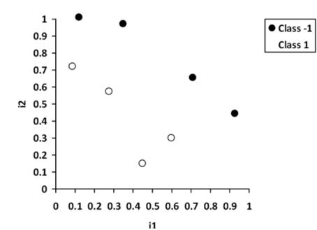
(a) It looks like there exists a perfect classification function for this problem that is linearly separable, and therefore a single perceptron should be able to learn this classification task perfectly. Let us study the learning process, starting with a random perceptron with weights w0= 0.2, w1= 1, and w2= -1, where of course w0is the weight for the constant offset i0= 1. For the inputs, just estimate their coordinates from the chart.
